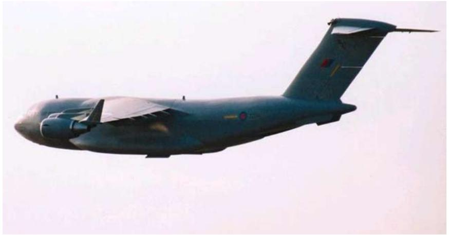
This 1/9th scale radio-controlled C-17 model was built in the United Kingdom for a 15 program series on the Home and Leisure satellite TV channel. Built in one year with the aid of three friends. Powered by 4 Jetcat P-120 turbines with a total thrust of 108 lbs. The model weighs over 250 lbs fueled. Wingspan is 20 feet 8 inches, and the top of the fin is 74 inches above the ground. The rear cargo doors open and they drop an r/c jeep on a pallet, as well as 2 free-fall r/c parachutists.
